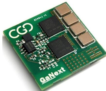
Prototype of a half-bridge module with CGD's 650 V GaN
